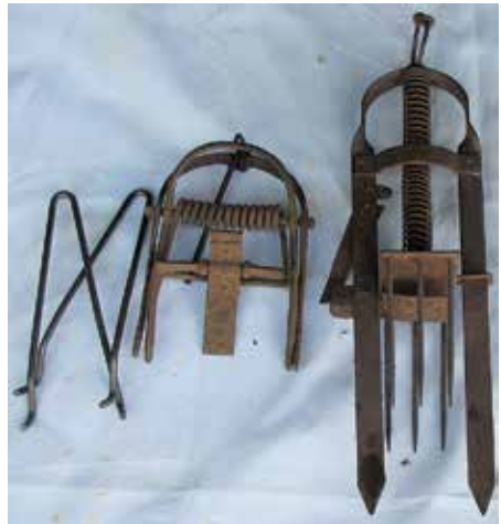
Fig. 8. "Out-of-sight" (left) and Harpoon (right) mole traps.
