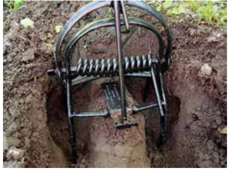
Fig. 13. Place trap in mole hole.
