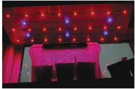
Fig. 5: A 0.5 m 2 homemade lamp fixture of 30 watts (see text for components).
